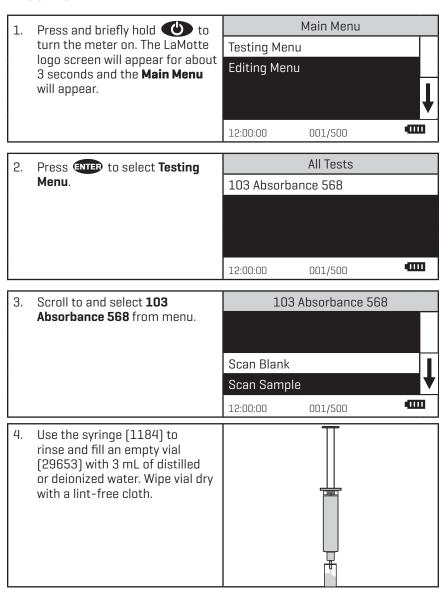
5. Insert vial into chamber, close lid and select Scan Blank. Use the syringe (1184) to rinse and fill the same vial with 3 mL of standard solution. Wipe vial dry with a lint-free cloth. Insert vial into chamber. Close 103 Absorbance 568 lid. Select **Scan Sample**. Record 1.350 result. Scan BLank Scan Sample 1111 12:00:00 001/500 103 Absorbance 568 Press V to scroll to 8. Calibrate. 1.350 ppm %T/Abs Calibrate Ш 12:00:00 001/500
